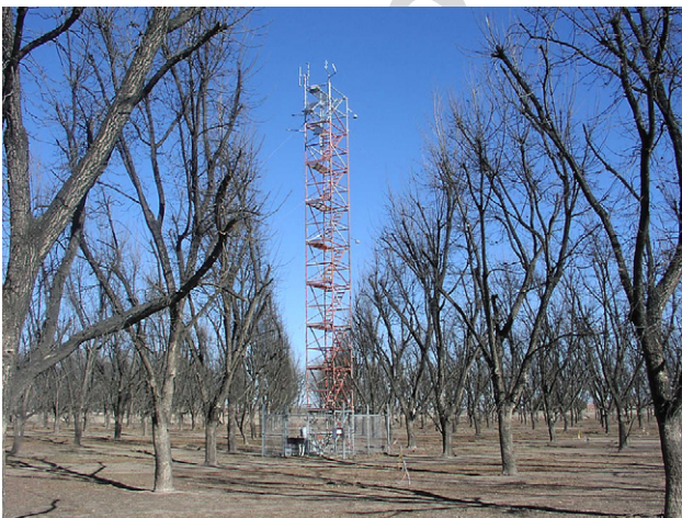
Fig. 1 – Eddy-covariance instrument tower in the pecan orchard in January 2003.
